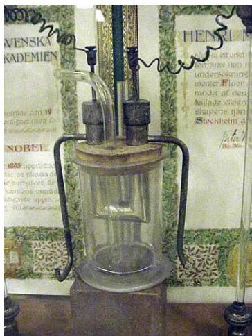
Figure 6. Moissan's Electrolysis Apparatus Used to Produce Elemental Fluorine, which Stands before His Nobel Prize Certificate at the Musée Henri Moissan, Paris. Photograph by James L.Marshall. (Courtesy, James L.Marshall)
